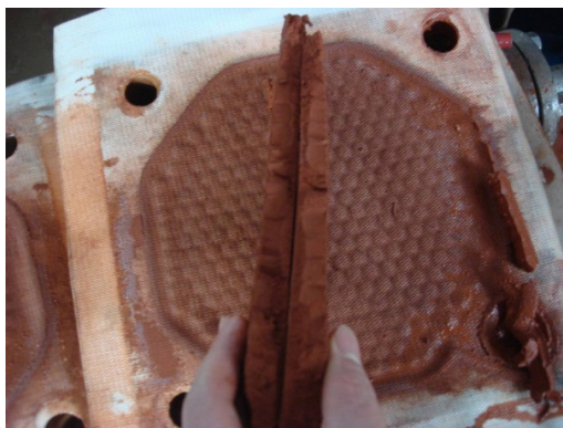
Figure 2. Press filtered reject (minus 37 \mu m fraction) at 75 % solids w/w.
