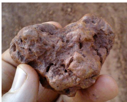
Figure 3. Roundness observed in an overscrubbed bauxite particle.
